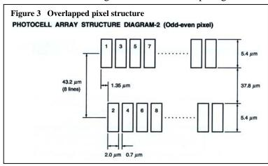
However the lens system must now magnify by 7.84 x (rather than 5.29 x) to fill the 8.5 inch platen and the effective pixel size become 21.6 um x 42.3 um and has X-Y asymmetry.
