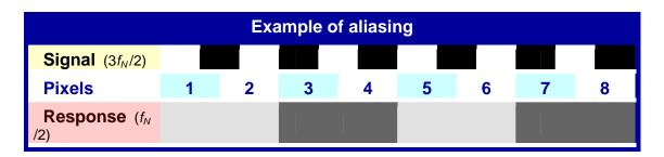
The first sensor null (the frequency where a complete cycle of the signal covers one sample, hence must be zero regardless of phase) is *twice* the Nyquist frequency. The sensor's average response (the average of all sampling phases) at the Nyquist frequency can be quite large.
