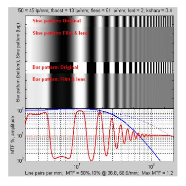
Figure 5. Illustrating MTF (courtesy of Imatest)
